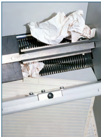
Automatic mechanical feeding system utilizes revolving flaps to feed material into cutting knives
